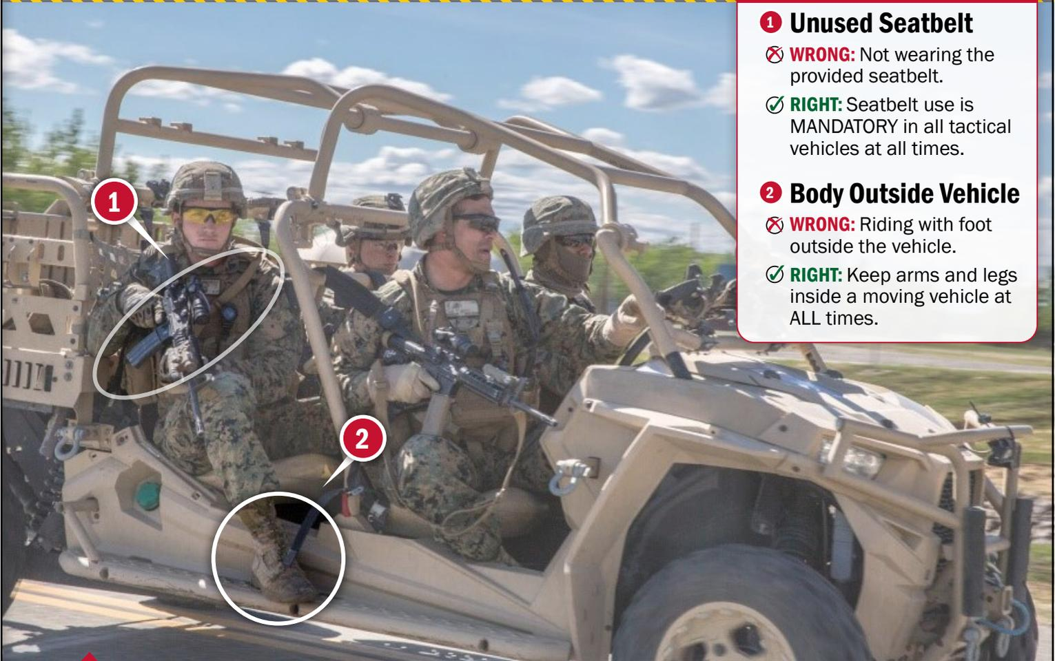
Operating the vehicle within its limits and observing mandated safety requirements will mitigate the potential for a rollover and minimize injuries if a rollover occurs
